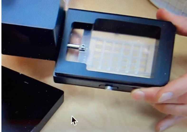
Figure 1. Multimodal tension device with stretch capacity mimicking both in tension and frequency, exercising native human skeletal muscles on a micropatterned 3D stretchable platform.
